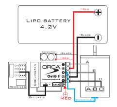
\* Install/Solder the relevant battery connector (Battery Specific) to the battery wires. Red to +ve and Black to -ve. (WARNING! Reversing the battery polarity will destroy
