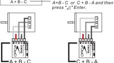
Use " "button and "▼"button to find the right Position of the motor link
